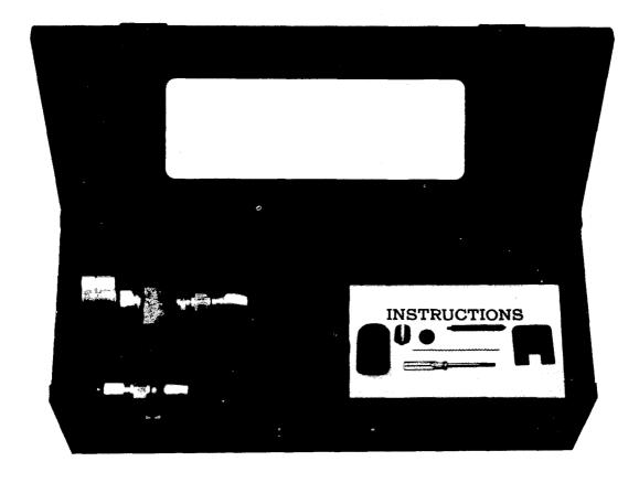
The instrument is pocked in the carrying case with the flexible hose disconnected. Unscrew the Jacking Out Nut, C-13 off the valve assembly. The instrument is then ready for use. It is connected to the engine cylinder by means of a suitable adaptor.
